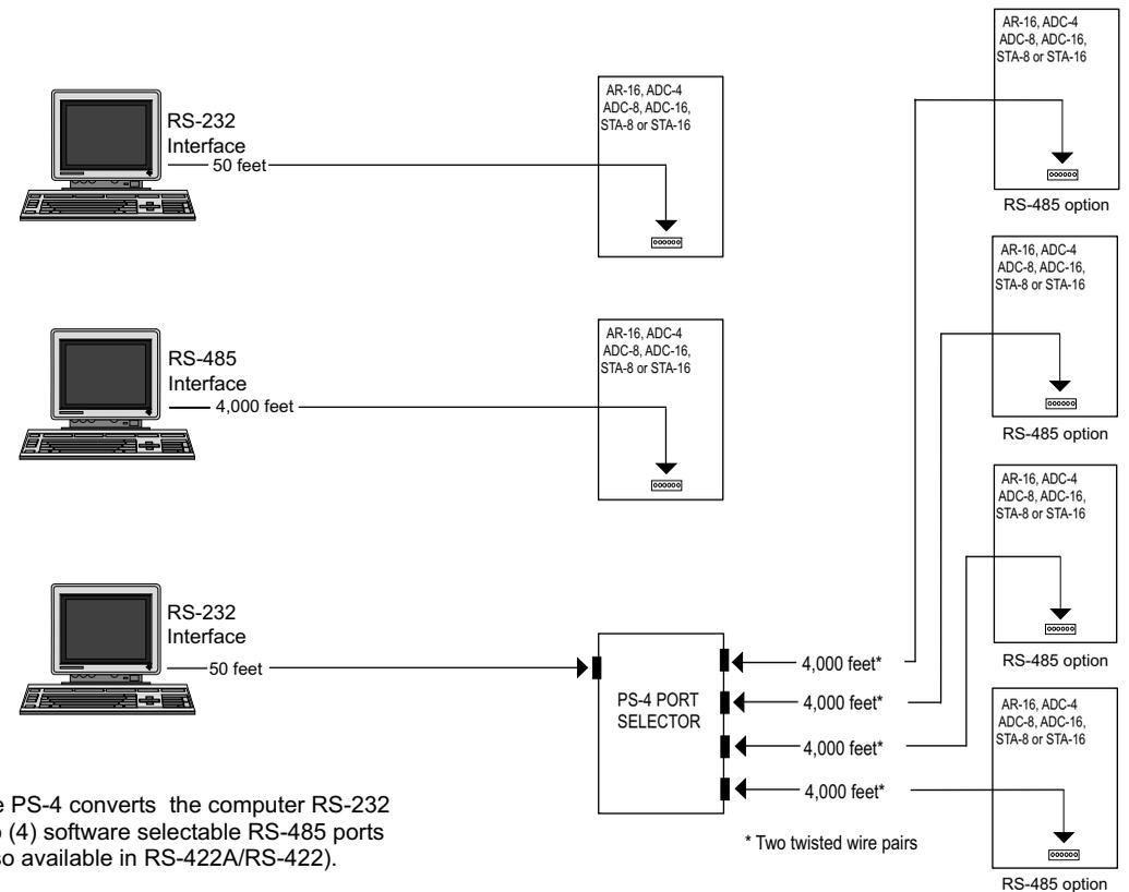
The PS-4 converts the computer RS-232 into (4) software selectable RS-485 ports (also available in RS-422A/RS-422).
