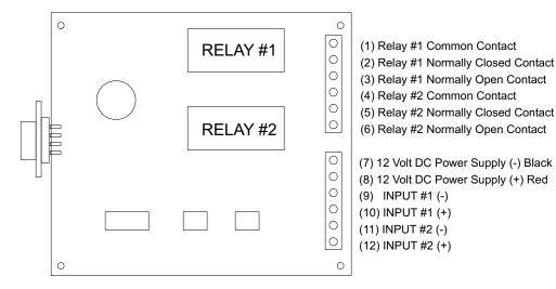
NOTE: The terminal assignments are also shown on the underside of the AR-2S Relay Interface. The RS-232 connections are made to the DB-9 connector on the AR-2S as shown on the following page.
