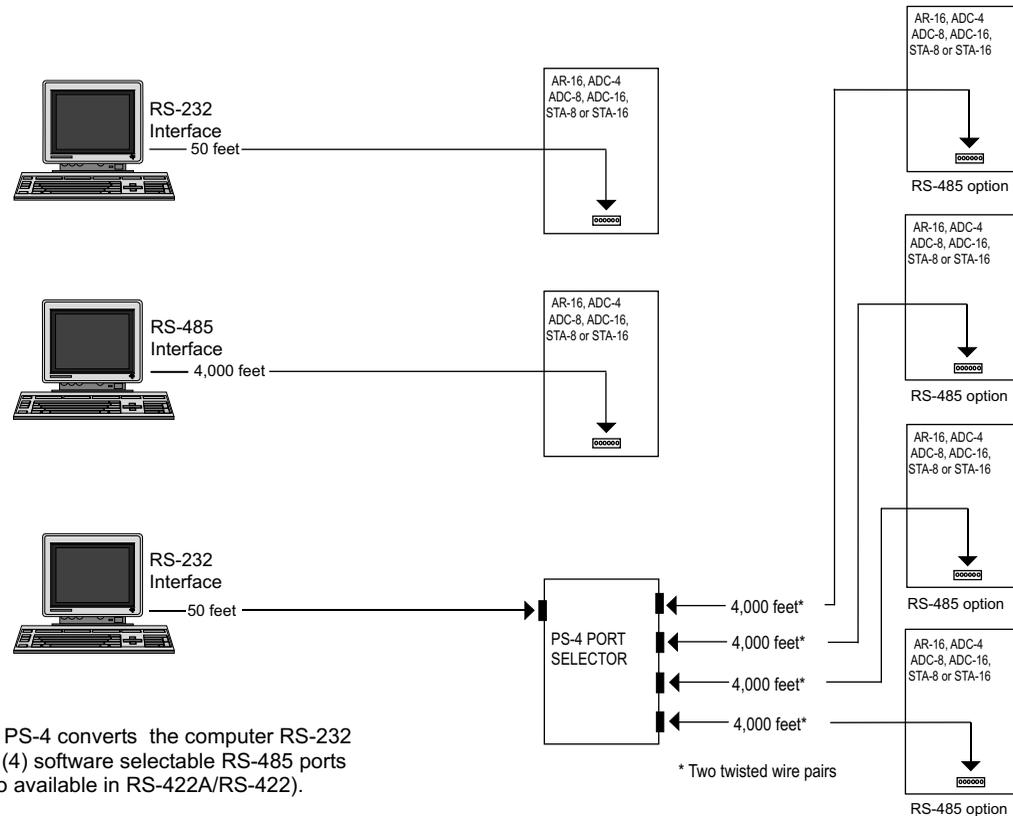
The PS-4 converts the computer RS-232 into (4) software selectable RS-485 ports (also available in RS-422A/RS-422).
