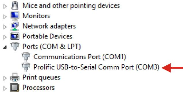
\*verify that this is the com port assigned to the ADC-12U12 by unplugging the ADC-12U12 (not hub) from your USB port and watching the entry in device manager. The entry should disappear and then reappear when you plug the ADC-12U12 back in.
