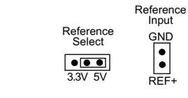
Shown to the right are the reference select and the reference input headers that are located by the terminal block on the ADC-4DU8. The reference select shows the shunt in the default 0 to 5 volt position. The reference select below shows the 3.3V position.
