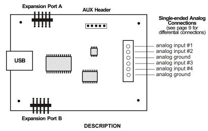
The ADC-4U series Analog to Digital converters connect to any available USB port on your desktop or laptop PC (including some tablets and phones). Four analog inputs channels are provided for conversion to 8, 10 or 12 bit digital format. The converters may be set to two channel fully differential mode if required. Three optional expansion ports are available for connection of up to 144 relays, 144 status inputs or combinations of relays and inputs.
