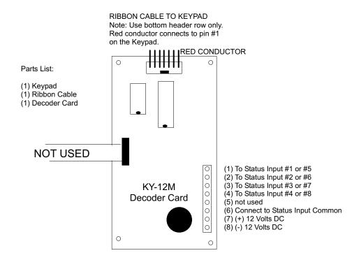
NOTE: Supply power to the KY-12M decoder by installing 2 jumper wires from the STA-16 or ADC-16 (+) and (-) to the KY-12M decoder. Connect a wire from terminal 6 on the KY-12M to terminals 9 or 10 on the RCT-8 to power the STA-16 or ST-32 opto isolators.
