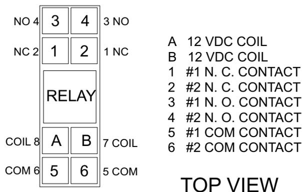
**IMPORTANT NOTE:** Connect HVAC equipment up to the N. C. contacts so equipment will operate with the relay in a de-energized state.
